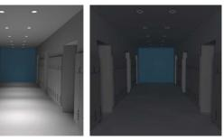
The presence detector can be adjusted in such a way that the lighting in an abandoned space will not switch off immediately after departure of the last
