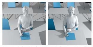
To ensure optimal conditions for writing it is suitable to place the luminaire for its luminous flux to be directed from above and moderately from the left hand side in the direction of the pupil's view. Using this solution the pupils do not cast a shadow when writing and good visibility of the pen point is ensured.
