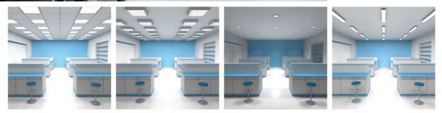
When selecting the luminaires for the labs and workshops it is necessary to take into account several factors at the same time. It is suitable to use luminaires with the protection level IP 54 or IP 65 in these spaces. In the workshops where there is a higher risk of injuring by moving rotating or reciprocating machines the luminaires should be fitted by electronic control gears to prevent the rise of the stroboscopic effect.
