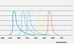
LEDs do not require colour filters. The colour tone of the light is determined by the semiconductor material used and the dominant wavelength.
