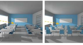
Direct glare can be prevented by correct organisation of the working plane. Placing the desks rectangular to the windows will prevent pupils to be directly exposed to the sunshine and thus to the undesirable glare.
