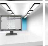
Indirect glare represents the same psychological and physiological burden as the direct glare. Moreover, it reduces the ability to perceive the contrasts. It is aroused by the disruptive reflection non shield luminaires. It arouses of light falling from the luminaires or unblinded windows from glossy surfaces (e.g. glossy paper or monitor).
