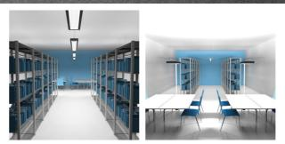
When designing the library lighting system the emphasis is laid also on the vertical illumination of the racks and shelves. The correctly illuminated racks ensure sufficient visibility of the books from the highest shelf to bottom one. The linear suspended luminaires with the direct and indirect radiation component, located along the aisles between individual book shelves are considered a suitable solution. The standard EN 12464-1 determines the minimal illuminance 200 lux for the racks.
