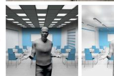
For the correct modelling of the faces it is important to ensure in the classrooms sufficient cylindrical illuminance amounting 150 lux. The suspended luminaires with the direct and indirect characteristic of the luminous flux distribution which eliminate forming undesirable shadows and at the same time do not cause glare are the optimal solution.
