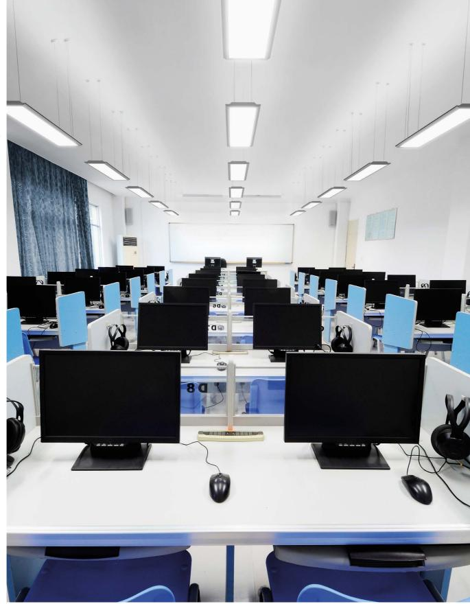
light sources and correct layout in the individual levels of the of the luminaires. In the rooms with availability of daylight it is due to the same reason to fit the windows with systems of curtains or blinds. The minimal shielding angles of the light sources and the value of the psychological glare admissible for the computer rooms are adapted by the European stand- lighting to the required intensity ard EN ISO 9241-307.
