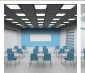
The recessed luminaires with louver with the direct characteristic of the luminous flux distribution are not suitable for the classrooms. We will not achieve the sufficient illuminance of the ceiling.
