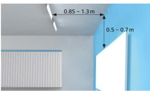
For illuminating the presentation surfaces we use most frequently the asymmetric luminaires placed 0.85 to 1.3 metres from the presentation surface.
