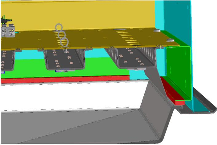
Corner detail to show C channel and led tray mount positions
