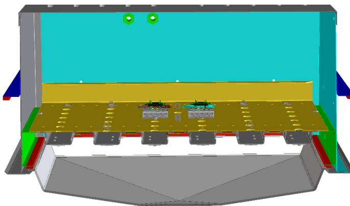
REXHP226LEDRET kit installed in to HEPA body. Gear Box is remote from body and not shown
